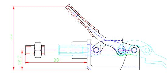
HANDLE OPENS 190° PLUNGER STROKE 16.7mm
